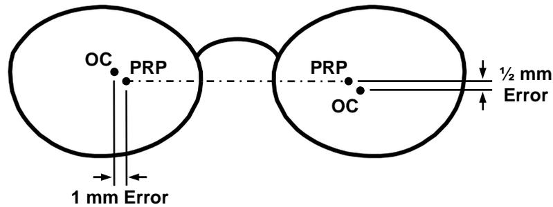
**Figure 5 – Horizontal and Vertical Prism Tolerance Markings**
