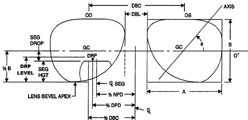
Figure C.1 – The Boxing System of Measurement
